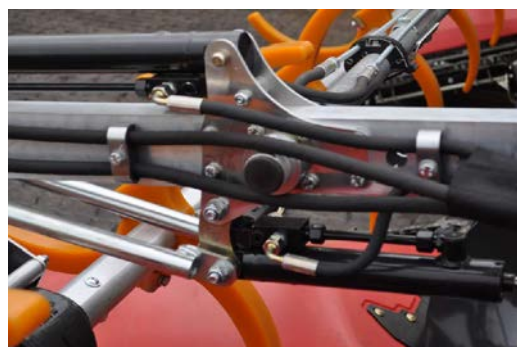
Hose lines to the hydraulic motor
