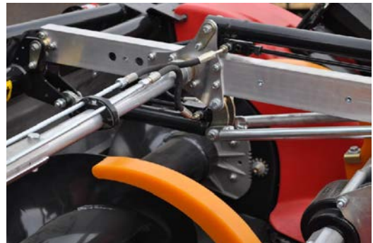
Pipe line, horizontal and vertical adjustment
