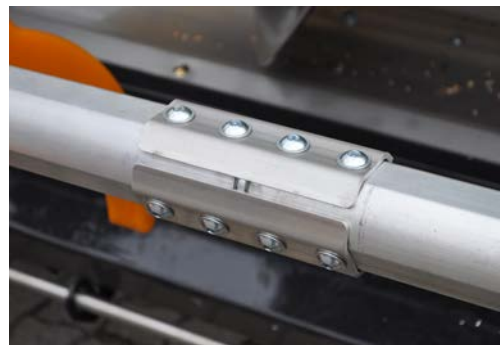
Connectors on profile pipe
