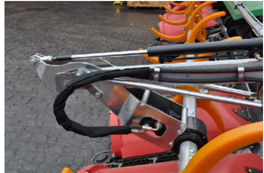
Line to the hydraulic motor and cylinders
