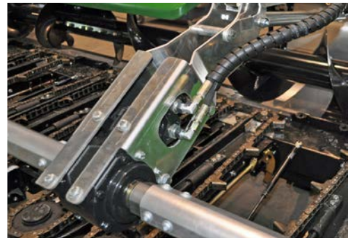
Hydro motor connection
