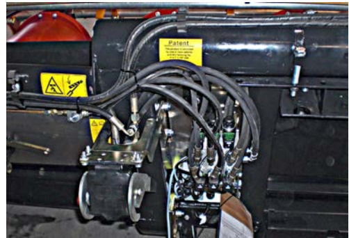
Hydraulic valve on the LH side of the machine frame
