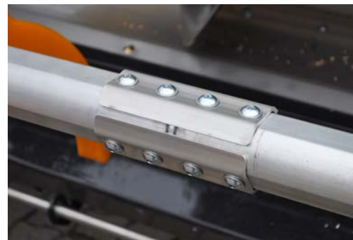
Connectors on profile pipe
