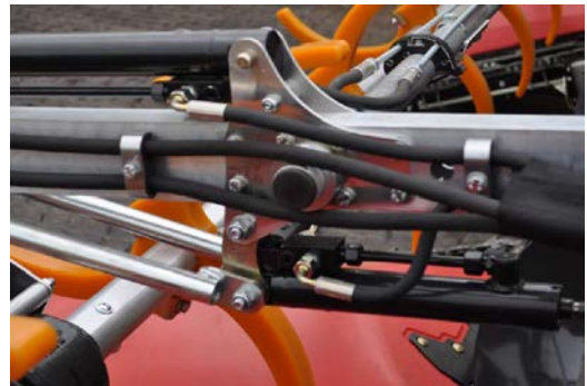
Hose guide at the end of the support arm
