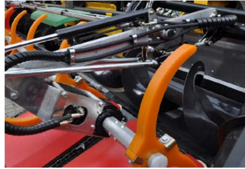
Hose clamps pre-installed
