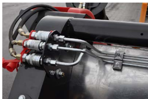
Pipe line to LH corn auger
