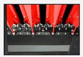
The SunLite cutter bar features the prestigious and durable Schumacker cutting system. Sickles are securely bolted in place for easy maintenance and can be replaced individually. There is no need to remove the entire bar during routine maintenance.
