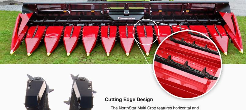
The NorthStar Multi Crop features horizontal and vertical gathering chains to allow harvest material to be transported steadily and safely to the thresher. All chains feature 12 posi-loc lugs for increased crop flow and the vertical conveyer chains are hydraulically driven and adjustable in speed. The chains work in unison to eliminate overloading, and reduce trash and build up for a smooth transfer of your crop.
