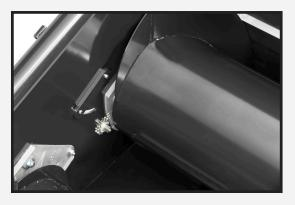
The SunLite auger can be easily adjusted to maximize crop flow. Adjust the gap between the auger and trough to accommodate your specific field conditions.
