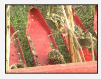
The durable chutes are spaced 9 inches apart and are integral to the grain pans. These pans reliably collect the sunflower heads and seeds that become dislodged then quickly transfer crop to the auger trough. Reliably decrease shatter and maximize your yield with the SunLite by Geringhoff.
