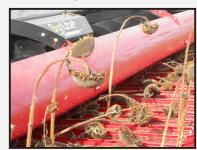
Designed with the ideal profile, the deflector allows the safest and gentlest way to assist crop towards the feeding roller. The SunLite's crop deflector cover can be quickly adjusted for ideal height and distance from the roller.
