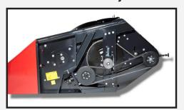
Both the main auger and feeding roller feature reliable drive systems with integrated slip clutch protection for peace of mind.
